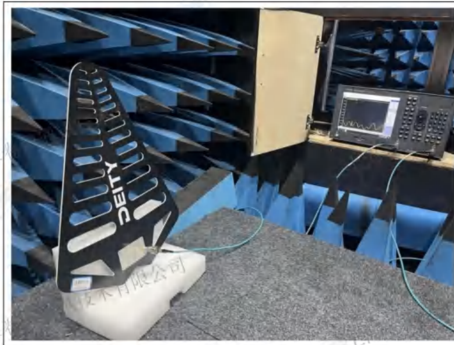
241018002 (WL-CT338板材天线) -电压驻波比测试现场图
